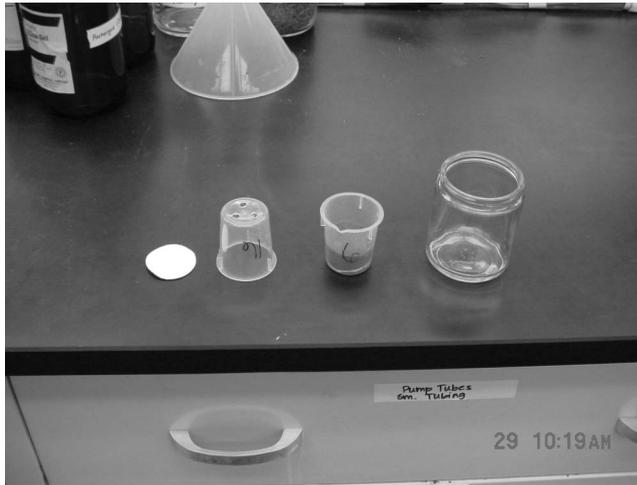
**Figure 6.** Materials for rewetting dry soil with capillary technique.
